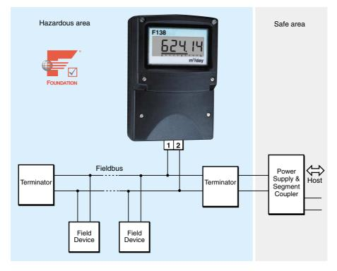
The BA414DF-F Fieldbus Indicator is a new cost-effective intrinsically safe field mounting instrument that displays a single fieldbus process variable in a hazardous area. Housed in a robust IP66 GRP enclosure, the instrument has a large, high contrast five digit display, plus a horizontal bargraph. The BA414DF-F indicator uses the same technology and compliments the well established BEKA eight variable fieldbus displays that are now in worldwide use.
